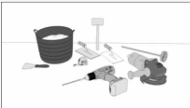
**I- Required material for installation:** a series of materials and tools are required, such as a notched trowel, a rubber trowel, an agitator, a level, a rubber mallet, a circular saw, meter markers, a spatula and adhesive paste.
