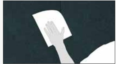
**7- Once the sheet has been installed, it id very important to take out excess of adhesive right away to avoid leaving debris in the surface. Clean thoroughly with a damp cloth or tissue and allow to dry.**
