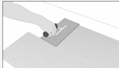
**The adhesive is applied with an adequately-sized notched trowel depending on the format of the piece to install.**
