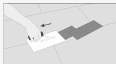
**The grouting material is applied with a hard rubber trowel, passing it repeatedly crosswise over the joints.**
