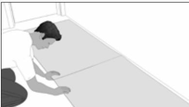
**2- Before installing, the floor shall be protected with cardboard or plastic to prevent staining.**
