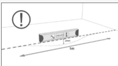
**It shall not have defects in its flatness larger than 2 mm, checked using a 2 m ruler.**
