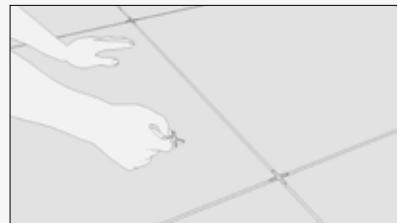
**A good tile installation and correct alignment requires using nylon spacers in order to leave open joints.**
