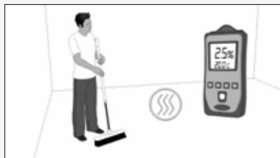
Substrates shall be completely dry (residual moisture shall not exceed 2.5%), stable, solid, resistant to compression, sufficiently leveled, and free of dust, grease, wax, paint, stripping agents, and anything else that could hinder adherence.
