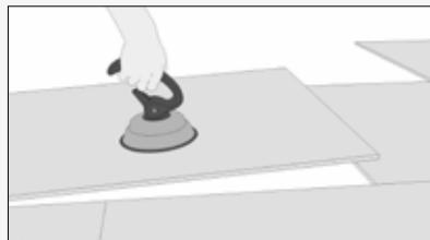
**We recommend that large tiles be installed with the help of a suction cup.**
