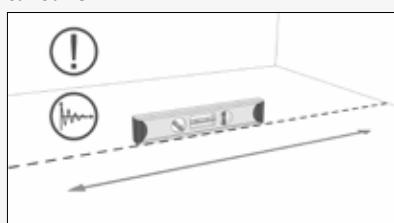
We shall verify that the substrate is vertically aligned, properly leveled, and it shall not have defects in its flatness larger than 2 mm, checked using a 2 m ruler.
