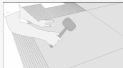
**To ensure contact with the substrate, it is advisable to lightly tap the tiles with a rubber mallet, in order to avoid the formation of air bubbles and gaps.**
