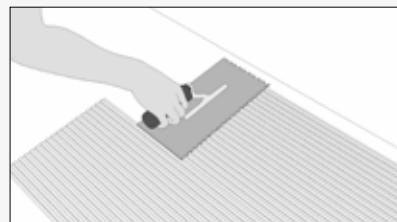
**We recommend applying the adhesive SUPER ONE+ UNILAX with a notched trowel, making sure that the amount spread over the substrate covers at least 80% of the DQS tiles.**
