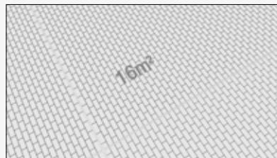
**Both perimeter and expansion joints shall be 10 mm wide, and we shall not leave a surface area greater than 16 m<sup>2</sup> or 8 m lineales without an expansion joint.**
