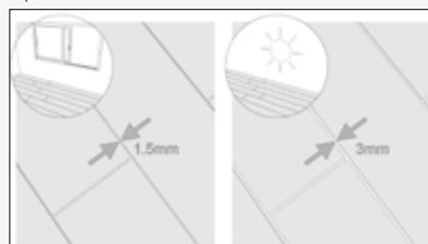
**It is very important not to install the tiles in contact with each other. We shall leave joints of a size that is adequate and proportional to the dimension of the piece. We recommend a minimum joint of 1.5 mm indoors, and a minimum joint of 3 mm outdoors.**
