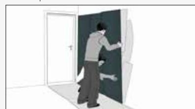
**6- Repeat the process with the rest of the sheets until they are all installed. You do not need to leave any joints, as the sheets are installed side by side. If you wish to seal the joints, we recommend to protect the sides of the edges with masking tape to avoid to stain the material with the joint sealer.**
