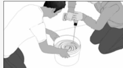
**5- Installation using adhesive paste. You must use a type R2 T two-component adhesive (EPOTECH from Butech recommended) and must mix well before application. Spread an even layer of the adhesive over the whole surface with a trowel. Once the adhesive spread, install the sheet by hand and then use a rubber trowel or metallic hand roller to set it in the right position and to avoid air bubbles.**
