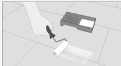
The protector is applied undiluted, using a thin foam roller, applying two crossed layers directly on the pieces. Only one application is required. Allow to dry completely.
