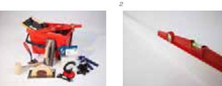
1 Installation of ceramic tiles should be carried out by skilled personnel, with demonstrable experience and appropriate tools and equipment, (i.e. toothed trowels, tile spacers, rubber mallets and suction cups for installation, and rubber trowels, sponges and containers for grouting). Check the information contained on the packaging beforehand, and meticulously follow the manufacturer's recommendations.
